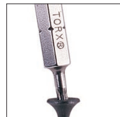
Wide tolerances can result in a loose fit between fastener and tool bit
