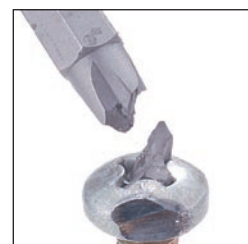
Concentrated stresses can cause breakage
